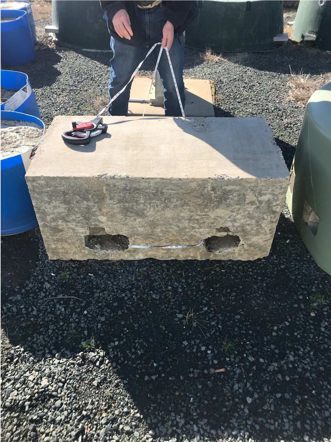
Figure 13: Concrete block - weights for 15m mast - 3m strop
